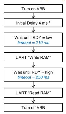
Note 1: Initial delay is needed for turning on VBB regulator, external switches and then establishing pull-up on RDY. If a slow external switch is used then this delay will be necessary to increase.
