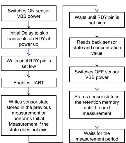
Measurement period of the sensor is determined by customer host system and may vary without degrading measurement accuracy.
